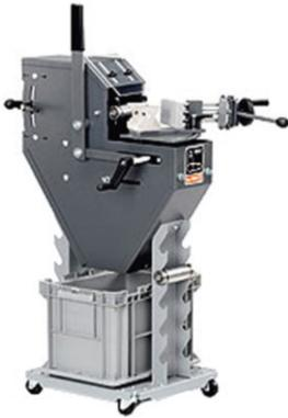
Grinds all angles between 30 & 90 degrees, Various size rollers are available. The unit is ideal for pipes and profiles of dia. 16 – 75 mm. Revolutionary speed of 1.500 rpm is ideal for VA-less heat, paint and burr pipes. Quick clamping for round and square tubes and flat material. With integrated adjustable depth stop, cross slide as standard equipment. The unit comes complete with one 75 x 2250mm, 36 grit belt and with one contact roller dia. 42,4 mm (1 1/4")
